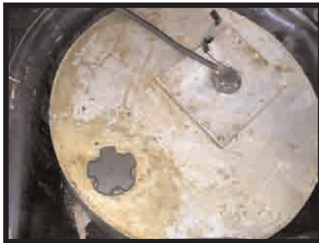
The vegetable tank that sits in place of the spare tire of Dave Lake's Volkswagen Golf.
